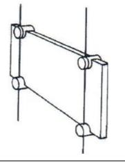
For the same use as the above except the panel is installed in front of the cables. No specific width required. **CS6.1 - Panel Support** Panel thickness Min: 4mm (5/32") Max: 8mm (5/16")
