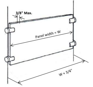
For this installation the panel is installed between the 2 cables. Ideal for enclosing areas, display panels, window display, etc.
